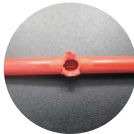
PAFSS fire suppression systems require no power for detection or operation. PAFSS fire detection tubing is installed throughout the risk area in the workspace, providing fast and effective detection of a fire. Upon flame impingement or high ambient temperature, the pressurised detection tube ruptures with a burst at the hottest point. The extinguishing agent is then discharged via the stainless steel pipework and nozzles which are aimed at the hazard area inside the workspace.
